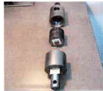
Fig. 4 — Setup for measuring under-head pressure prior to its installation in a load frame.
