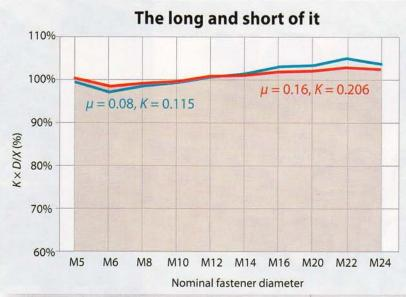
The short-form equation, T = K $\times D \times F$ , using an experimentally derived nut factor, K, gives slightly different results than the long-form equation over a range of fastener sizes as shown here for two different friction levels. Results fall within 5% of each other. The values for  $\mu$  and K were chosen to normalize traces for M12 fasteners.
