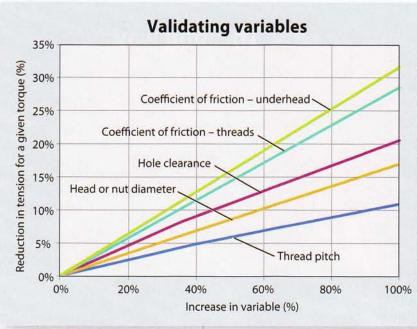
While the nut factor, K, in the short-form equation is experimentally determined, long-form equations use several variables to quantify the effects of thread pitch and friction on the torque-tension relationship. The traces shown here help explain the effect each variable has on bolt tension.
