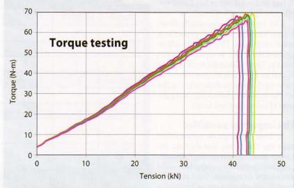
Torque-tension tests on simplified representative joints let engineers determine a nut factor that can define the torque-tension relationship for similar fasteners with different diameters. However, sample-to-sample variations in friction can make results vary by as much as 10%.
