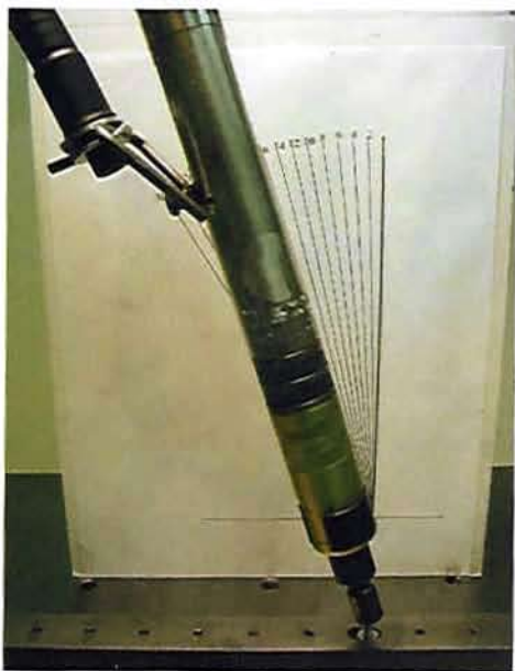
Figure 6.1.1 Test 3 setup. The flexible support shown to the left was used to assist the operator in maintaining an in-line orientation along the axis of the nut member.
